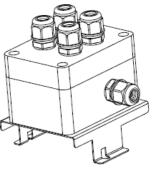
2. Let luminaire power cable pass through gland into junctionbox, and make wiring connections with AC power cable. Blue (N) : Neutral; Brown (L) : Line; Yellow/Green(G) : Ground
